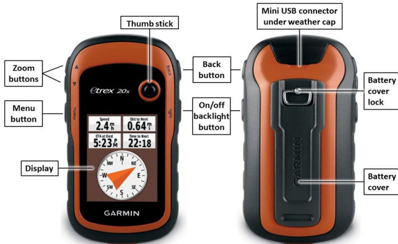
Figure 5.1 - Parts of the Garmin eTrex GPS device
